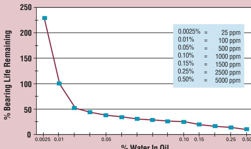
Effect of water in oil on bearing life (based on 100% life at .01% water in oil.)
