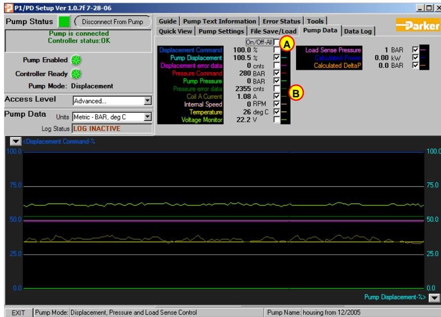
Figure 7: Pump Data screen of P1/PD GUI
