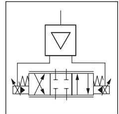
There is a linear relationship between the solenoid current and the input signal. The solenoid current is stabilized against voltage fluctuations as well as temperature dependent resistance variations of the solenoid coils. Because of the effect of load on the position of the valve spool, the spool position may vary and there is a limited relationship between the command signal and the valve flow.
