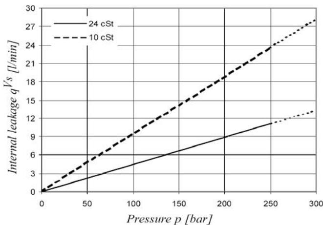
Do not operate pump more than 5 seconds at any speed or viscosity if internal leakage is more than 50% of theoretical flow.
